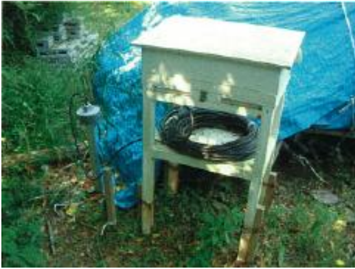
Figure 21 - Typical groundwater monitoring set up and schematic diagram of vibrating wire piezometer (after Indian Institute of Technology 2015)
