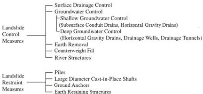
Figure 22 - Typical landslide mitigation measures (after Japan Landslide Society 2002)
